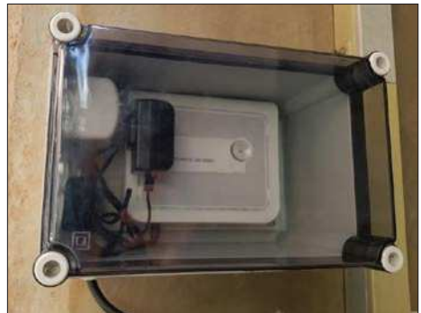
Fig. 2 – Avoid installing the power cable on top of the embedded antenna.
