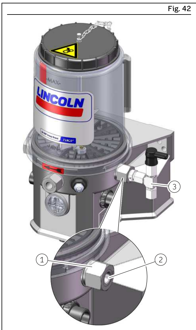
Replacing pump element and pressure limiting valve
